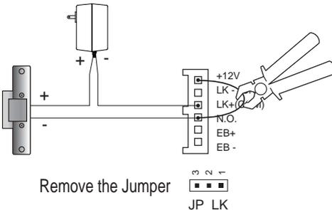
set to Normally Closed on the Unlock Relay mode
