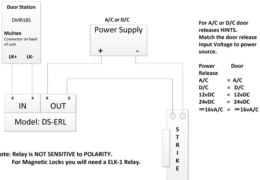
**Note:** Relay is NOT SENSITIVE to POLARITY.
