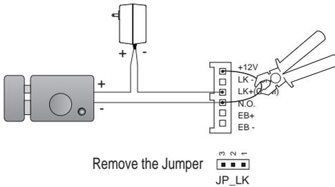
set to Normally Open on the Unlock Relay mode (default)
