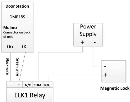
Power Supply can be A/C or D/C as long as it matches the needs of the magnetic lock.
