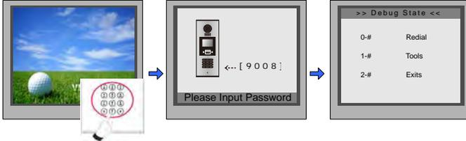
When door station is in standby, press '#' key Input '9008', then input the Admin Code.(66666666 by default) Debug state menu is launched
