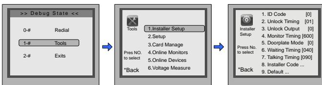
During working at debug state,press "1#" to enter tools page. Press NO."1" to enter Installer setup item. Installer setup page overview.
