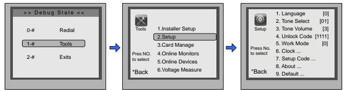
During working at debug state,press "1#" to enter tools page. Press NO."2" to enter Setup item. Setup page overview.
