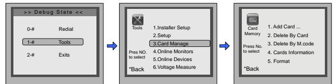
During working at debug state,press "1#" to enter tools page. Press NO."3" to enter Card Manage item. Card Manage page overview.
