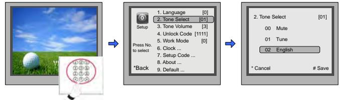
When door station is in standby, press '#8002'+code 66666666 to enter **Setup** page.
