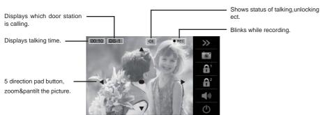
Note: The 5 direction pad operation should make in effect with fish-eye door station.
