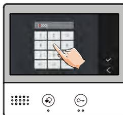
Step 4. Input number 8401~8499 to set the unlock time as 01~99 seconds.
