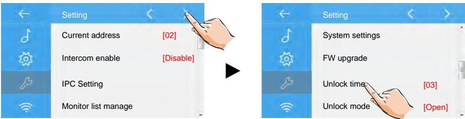
Step 3. The Installer Setup with keypad will show up. Then input number from 01-99 and touch OK to set the unlock time as 1-99 seconds.
