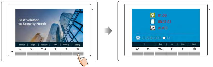
Step 2. When the screen stay in About page, press
