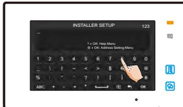
Step 4. Input number 8401~8499 to set the unlock time as 01~99 seconds.
